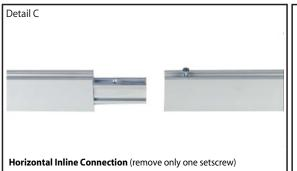
Remove only (1) setscrew when disassembling. Replace setscrew in extrusion after assembling it. Before packing, replace setscrew in extrusion to avoid losing it.
