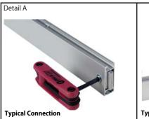
Most horizontal extrusion connections have a patented expandable lock. This lock inserts into the groove of an opposing extrusion. Tightening the lock with the Hex Key Tool expands the lock and creates a strong positive connection.
